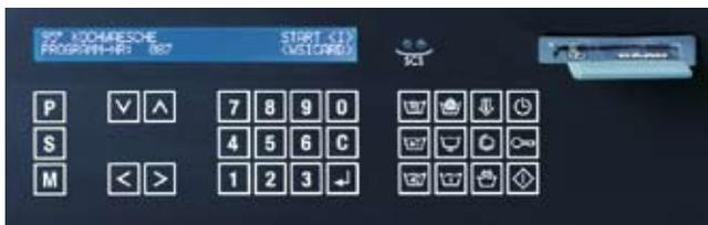
In addition, there are clearly arranged buttons. They follow the logic of the washing process and are identified with clear and explanatory symbols which correspond to common fabric care symbols. And all this in 8 languages.
